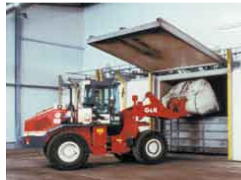
Filling of Herhof composting box through wheel loader
