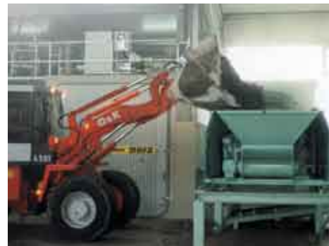
Processing of compost by means of screening technology
